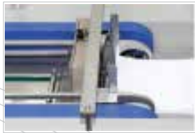
Dual automatic feeder Individual dual feeder for board and prints
